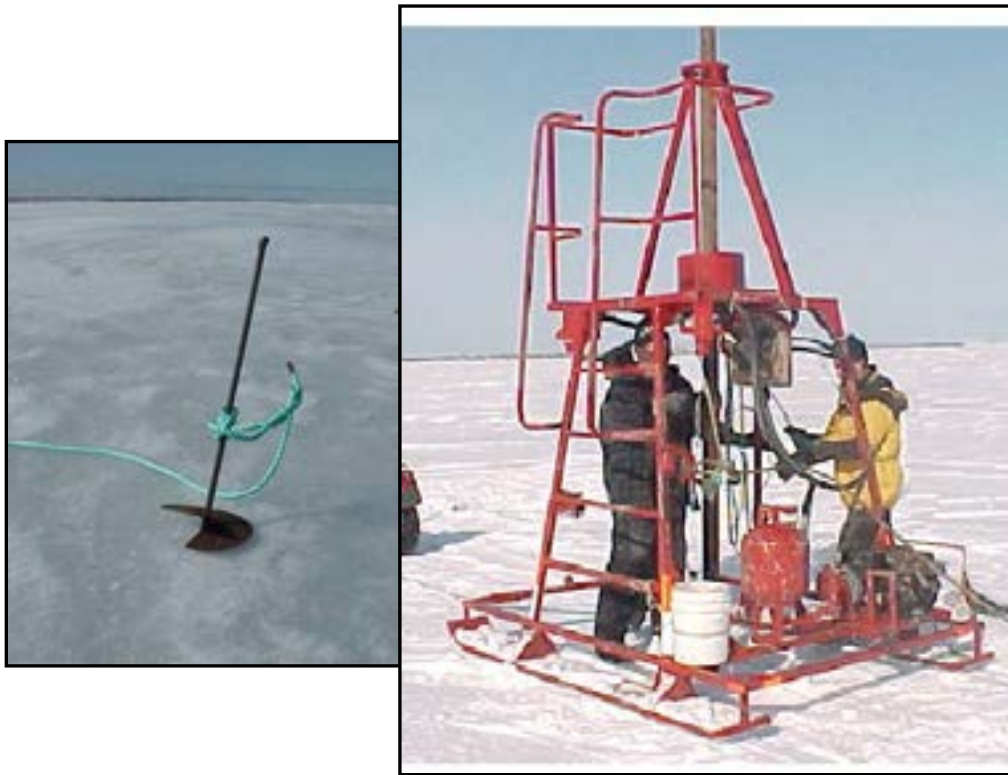
Figure 27 Helical screw anchor and hydraulic device
